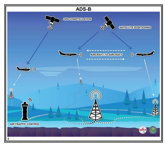
Automatic Dependent Surveillance-Broadcast (ADS-B) is a surveillance system in which an aircraft to be detected is fitted with a data link transmitter. The aircraft periodically broadcasts its Global Positioning System (GPS) – derived position, call sign, velocity, and other information over the data link. The information is received by a radio station for processing and display at an air traffic control facility.
